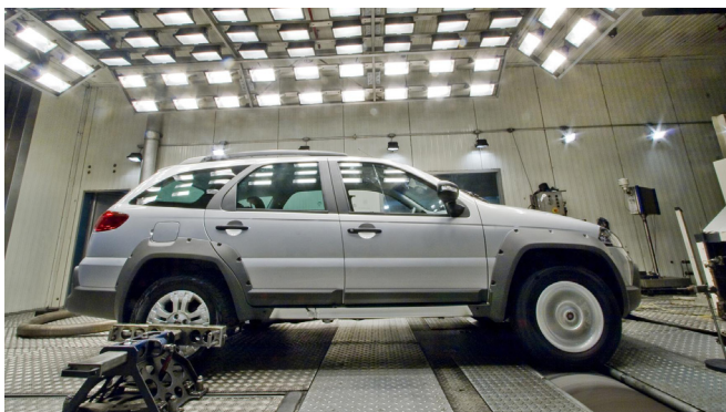
Figure 2 - Climate Chamber with Rolling Dynamometer Source: Fiat Press (2011)
